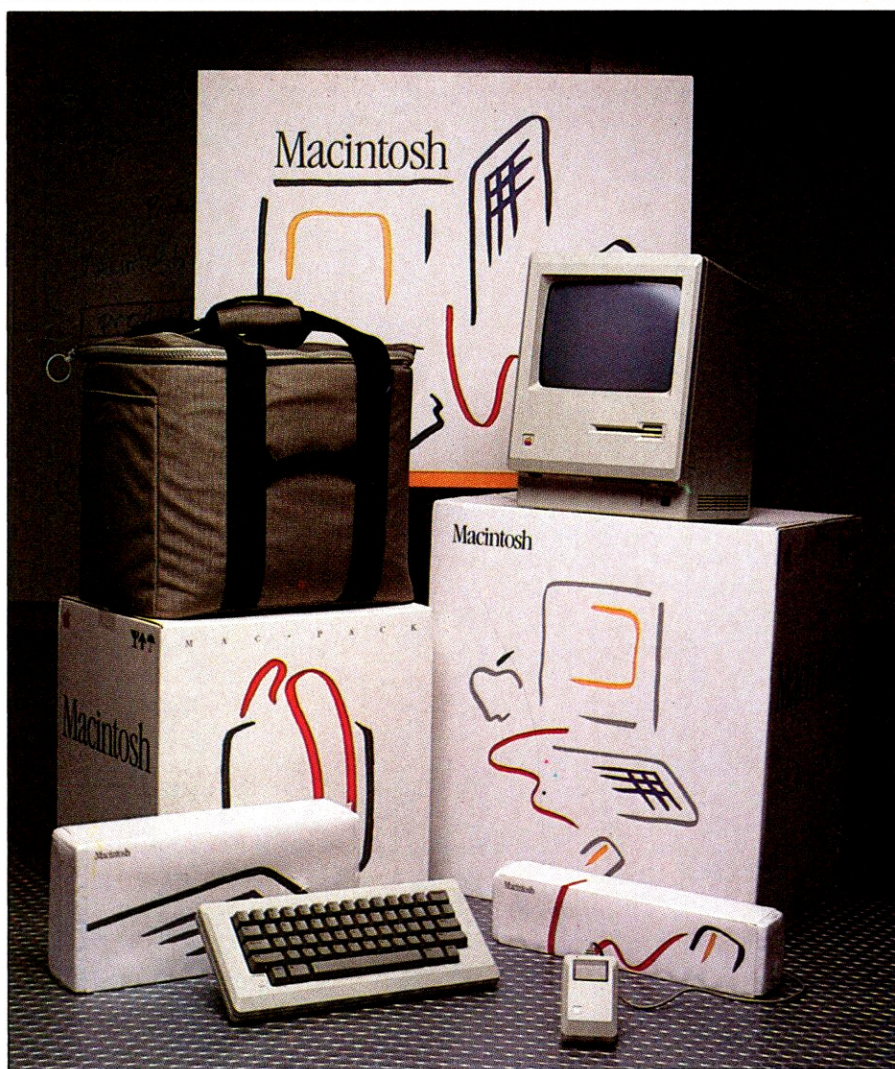
The system consists of a monitor, a 3½-inch disk drive, 128K of memory, a mouse, and a detachable keyboard.
